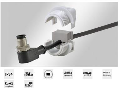
QVT is a circular split frame for quick and easy installation of pre-terminated cables or complete cable harnesses. But also electric, pneumatic or hydraulic lines without terminals or connectors as well as corrugated conduits can be easily routed and sealed with IP54. Because of its extremely compact design, the QVT range is especially suitable for small machines, devices and instruments.
